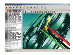
Renishaw's MODUS software includes a configurable user interface to allow native DMIS programs to be developed offline utilizing geometry, embedded dimensions and tolerance data from CAD.
